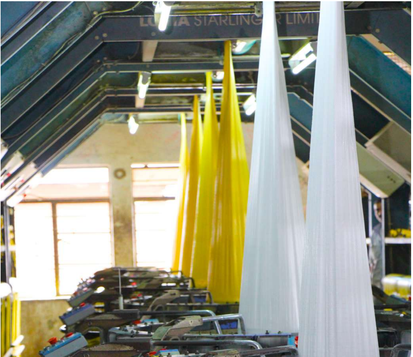
Circular Looms weaving fabric
