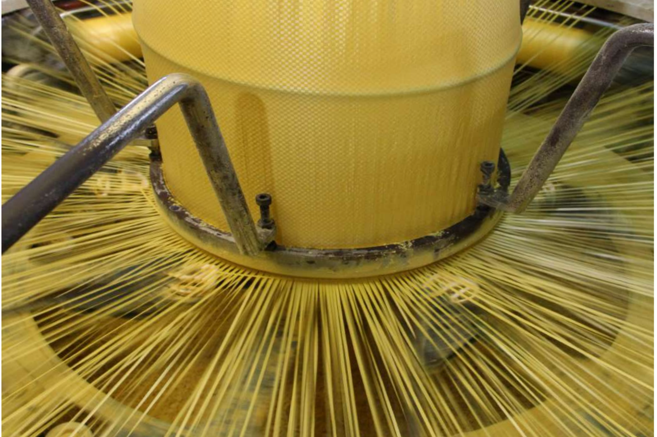
Circular Looms weaving fabric
