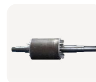
Copper Built up Rotor with Shaft inserted
