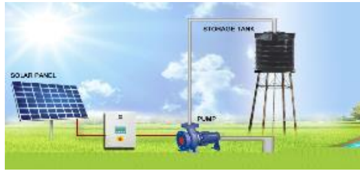
Solar Pumping System
