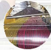
E-beam irradiated cables
