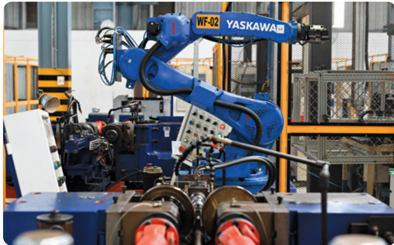
Motoman Robot conducts loading & unloading of component at the driveline
