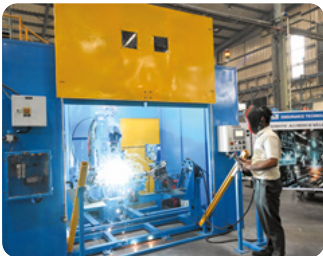
Robotic Welding system at the Aluminium Forging Plant
