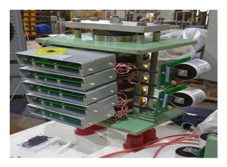
2. Successfully secured project for Electro Magnetic Launching System using 100mm SCR.
