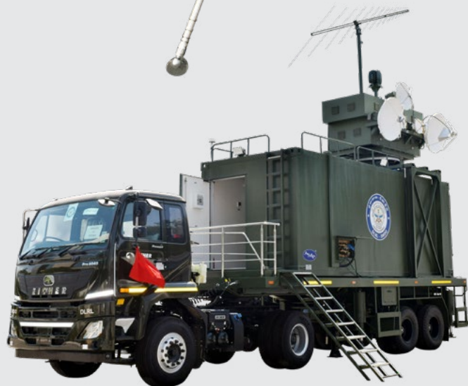
SRES: Radiation Mode Test & Evaluation facility for Radar EW Systems
