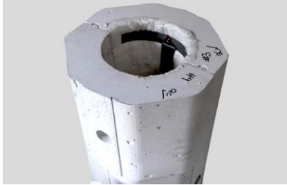
Precast Skid Pipe Cladding
