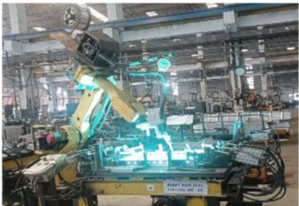
Robot at Mach one (Aluminium Welding)
