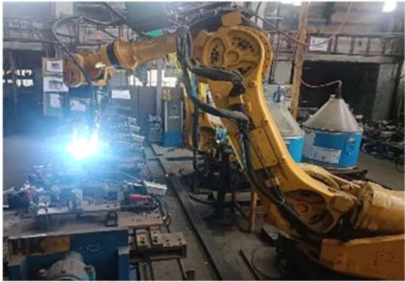
Robot welding at Scaffolding Dept.
