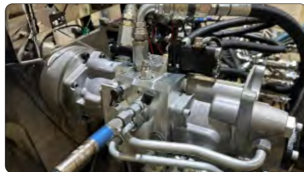
Newly developed Mobile Hydraulic System for Harvesters
