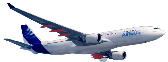
The Flap-Track-Beam Assemblies manufactured by Dynamatic for all Airbus aircraft are highlighted in red in the above image.
