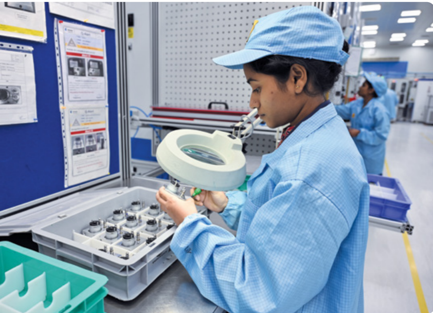
Q-gate inspection in Hydraulic Control Unit, ABS line
