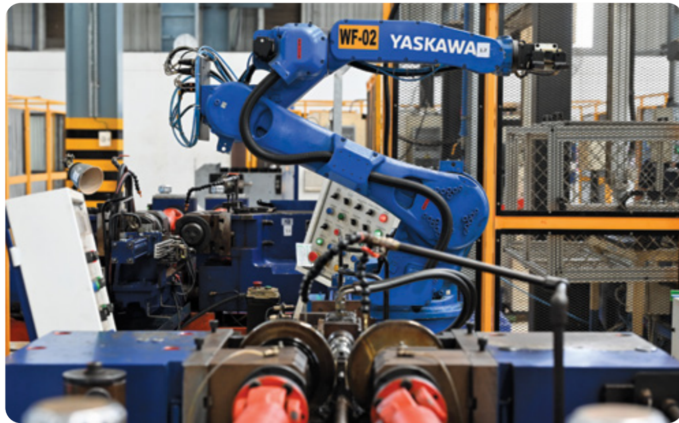
Motoman Robot conducts loading & unloading of component at the driveline
