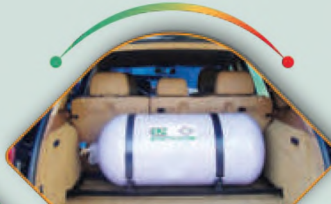
COMPRESSED NATURAL GAS CYLINDERS
