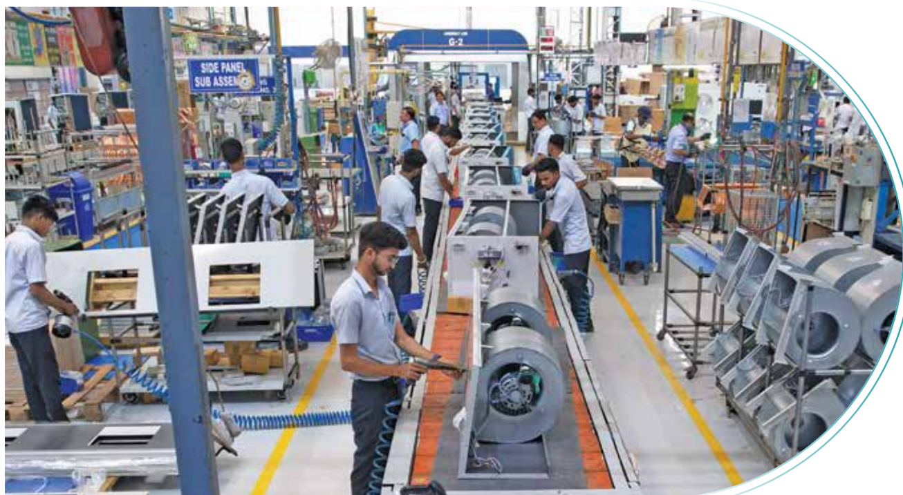
Dadra Plant's assembly line for ducted air conditioners
