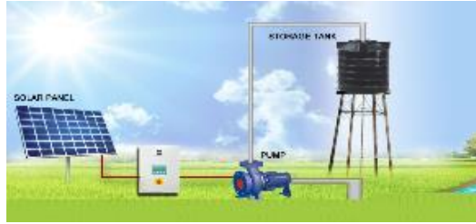
Solar Pumping System
