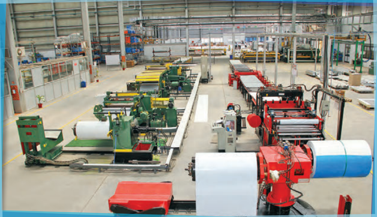
Sheet metal cutting at the fabrication unit at Blue Star's Wada Plant
