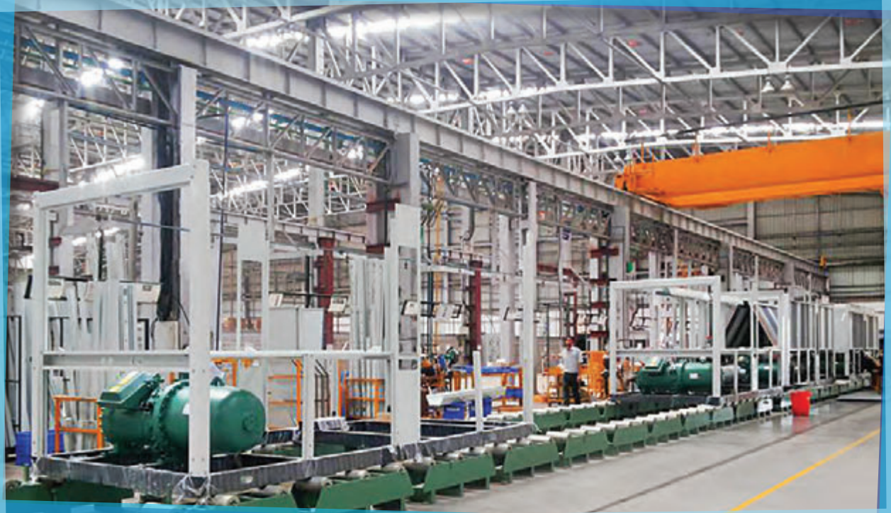
Screw chiller assembly line at Blue Star's Wada Plant
