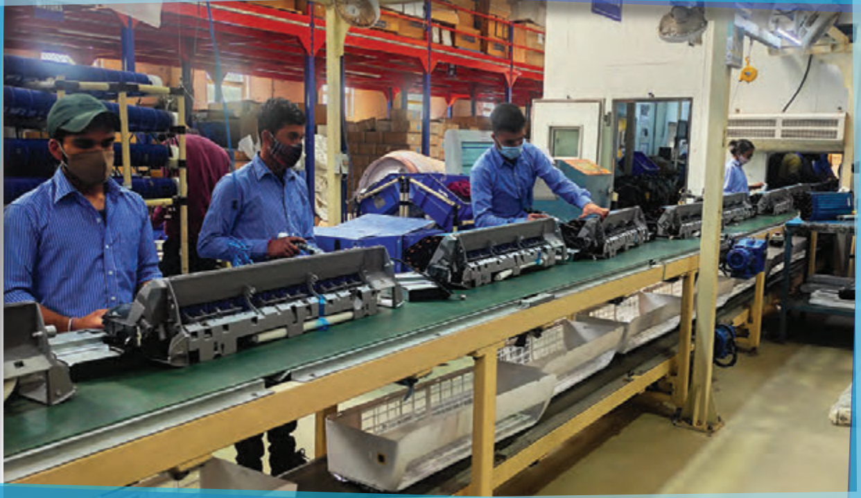
Indoor Unit manufacturing assembly line at Blue Star's Himachal Pradesh Plant
