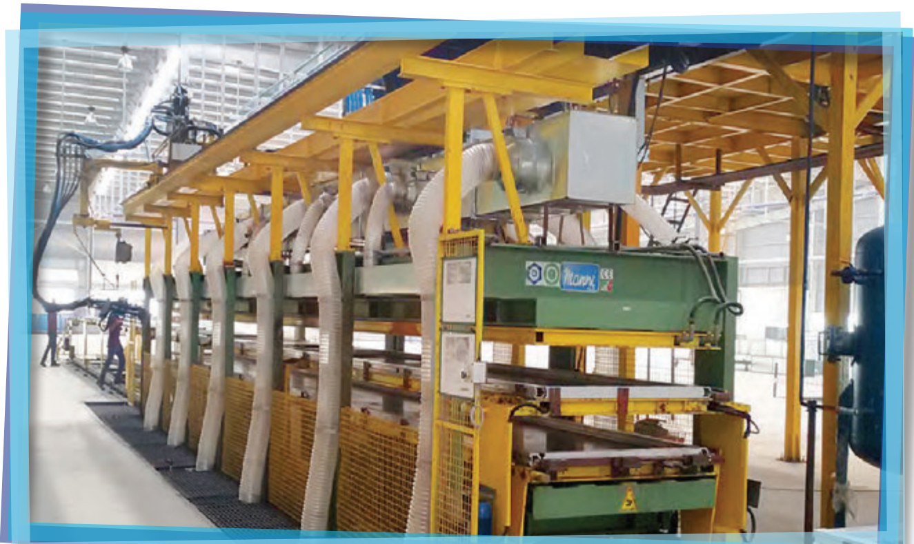
Foaming press cold room panels at Blue Star's Wada Plant
