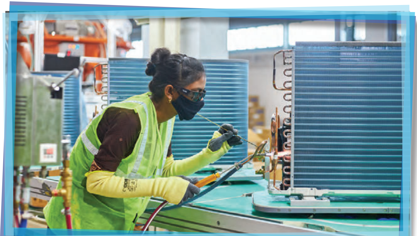
High Wall split air conditioner being manufactured at Blue Star's 100% subsidiary Blue Star Climatech Limited's Sri City Plant
