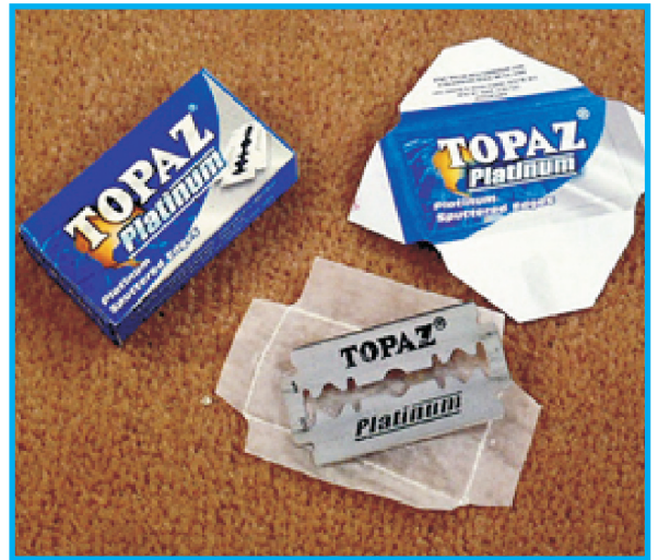
ANTI RUST TISSUE (Wrapping of steel, silver items and Razor blades as paper has anti- tarnishing properties)
