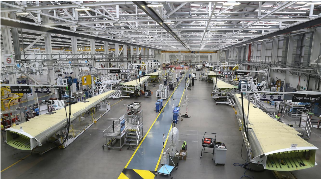
Airbus A220 wing assembly at Spirit AeroSystems' Belfast facility in Northern Ireland.
