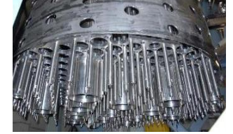
Control Plug for Reactor
