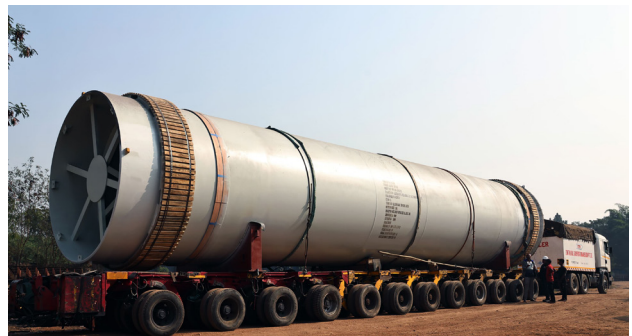
Rotary Kiln with Heating Jacket for a leading Fluorochemicals manufacturer in Italy
