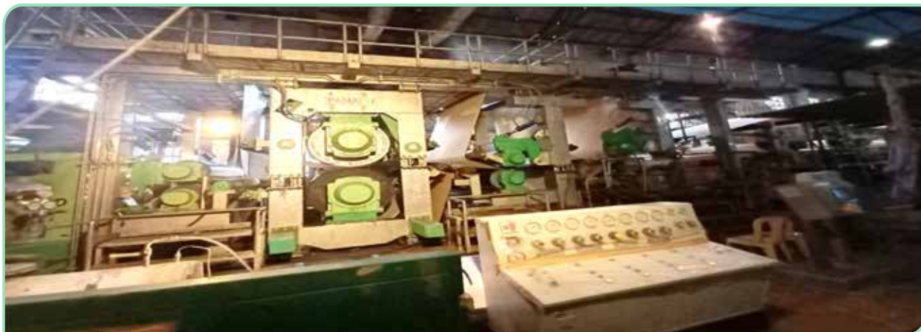
PM-5 REBUILD- NEW SUCTION PRESS ROLL
