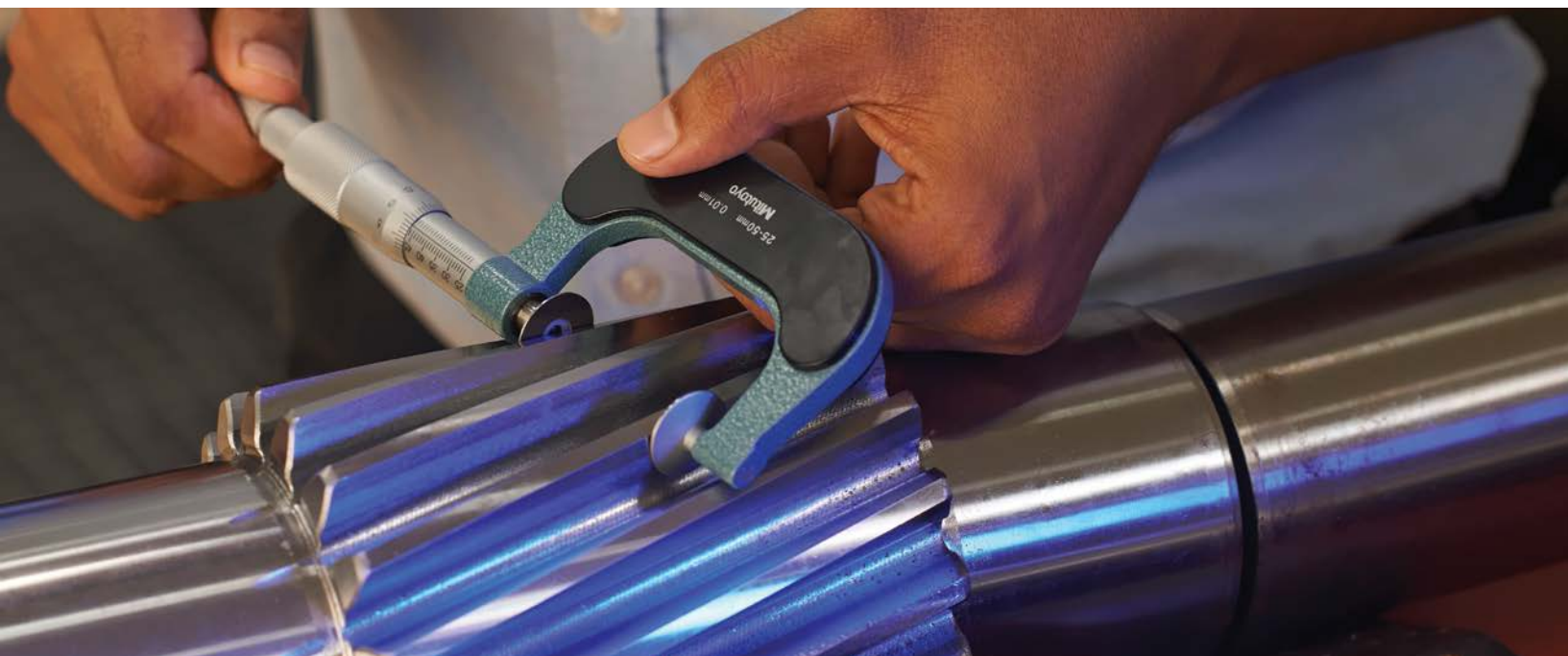
▲ Gear teeth dimension measurement by disc micrometre
