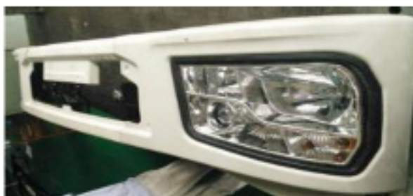
Bumper and bumper bracket: GFPP-L30/40/50, alternative metal, sprayable
