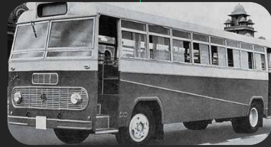
FRONT DOOR FRONT ENGINE
