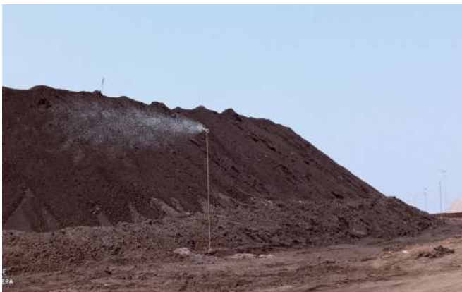
Spray Guns in Bunker Area
