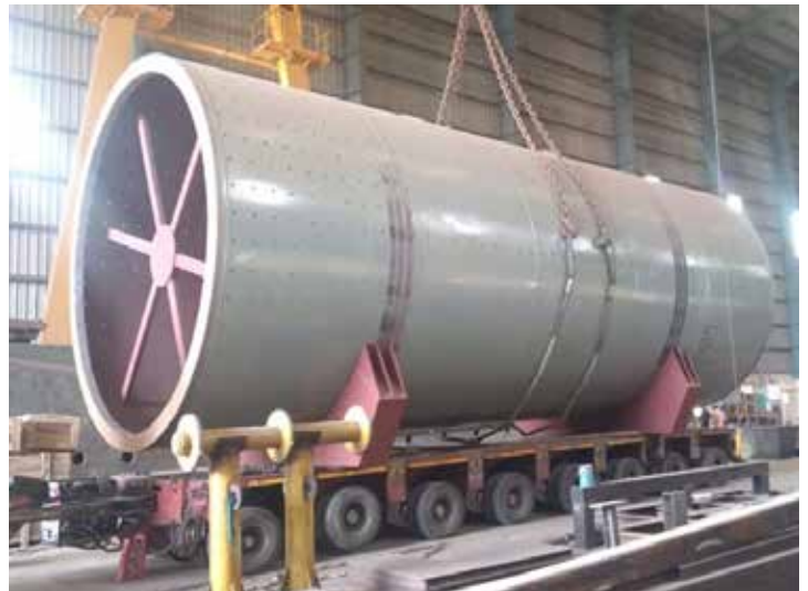
Mill shell for Volta Impex (Export Order): ID 5m X 12.39 m length X 40 mm Thick (72 MT)
