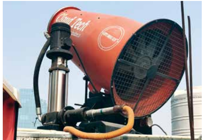
Anti-Smog Gun for dust suppression at Mahindra Luminare
