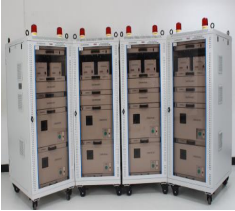
ADS-B receiver system for Airports Authority of India (AAI)
