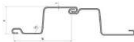
Z' TYPE SHEET PILES TYPE - B
