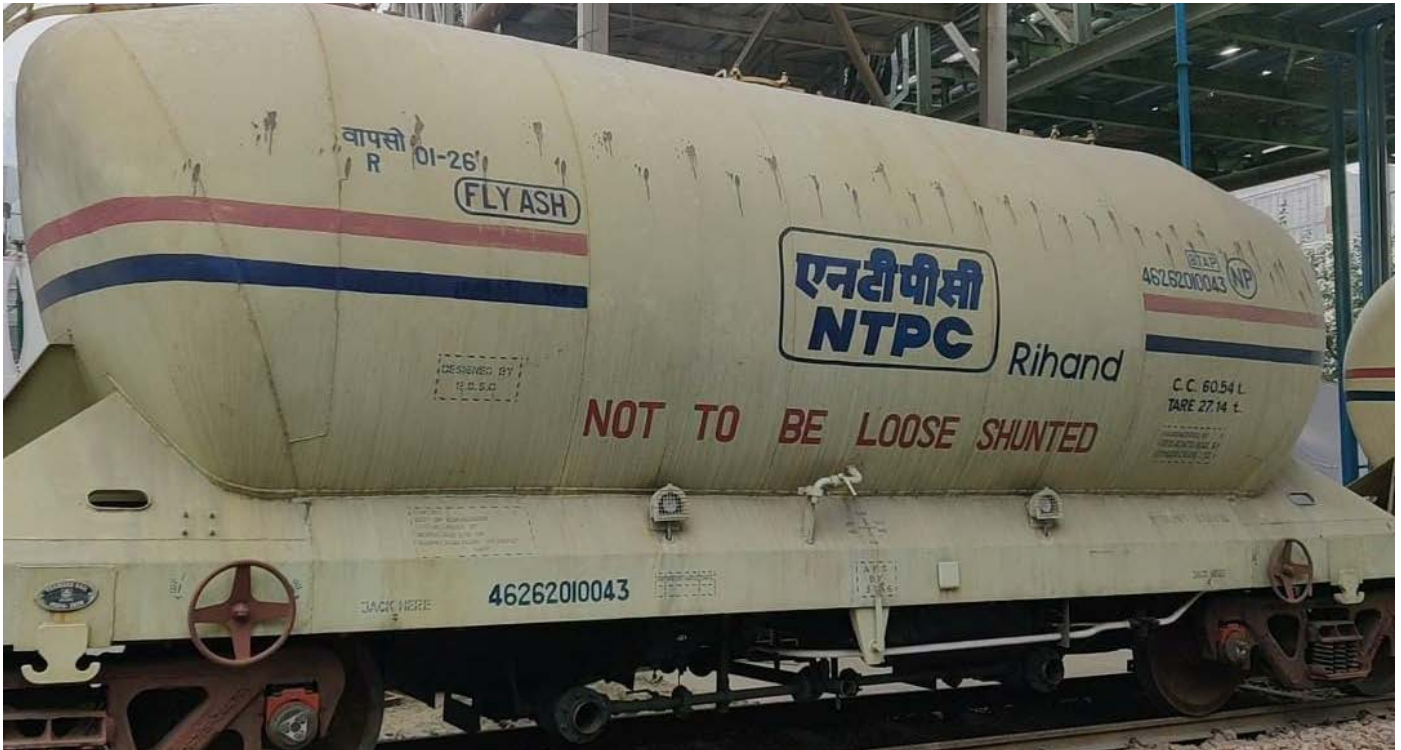
Ash Transportation through BTAP wagons
