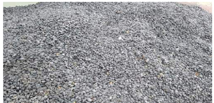
Ash based Geo Polymer Aggregate developed by NTPC
