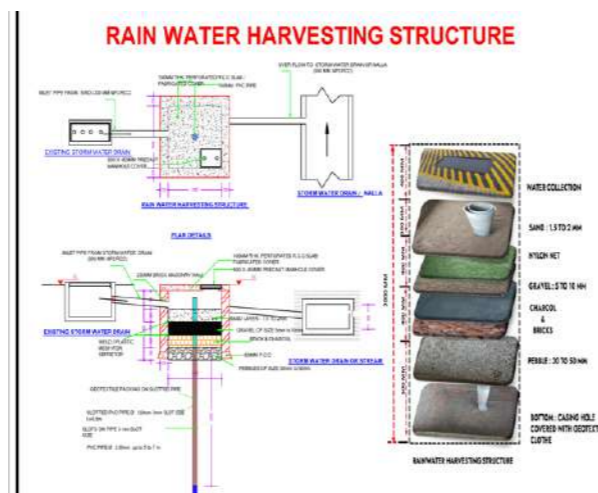
Conceptualized schematic depicting the Recharge Injection bore well & pit
