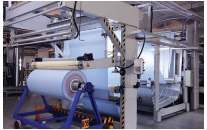
A view of Stenter Machine installed at our newly established Fabric Processing Unit.
