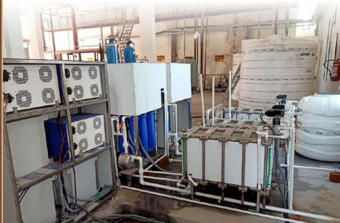
24 TPD Electro-Dialysis Reversal (EDR) Plant, NETRA
