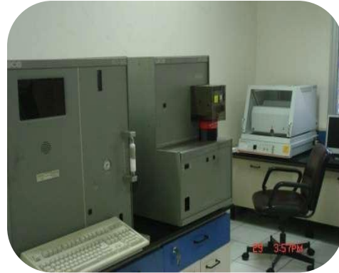
Leco Oxygen Analyzer: R0300 & X-Ray Fluorescence Spectrometer
