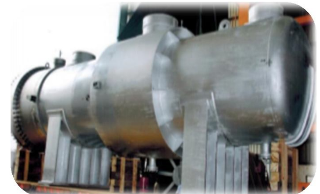
Moderator Heat Exchanger
