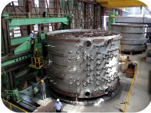
Calandria, 700 MWe Reactor
