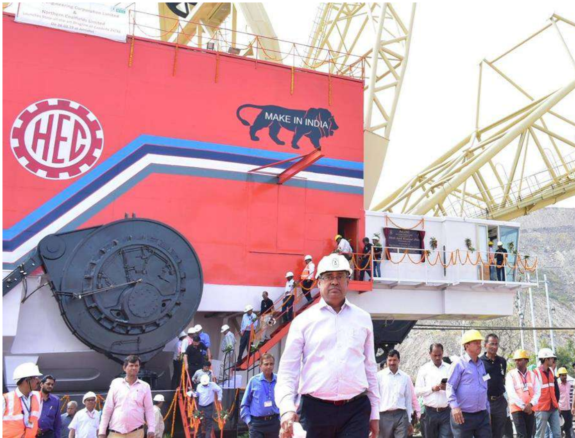
Fig. 4- Commissioning of “Agnee”, a giant Dragline with 24 cubic meter bucket capacity and 96 meter boom length, at Amlohri OCP, NCL
