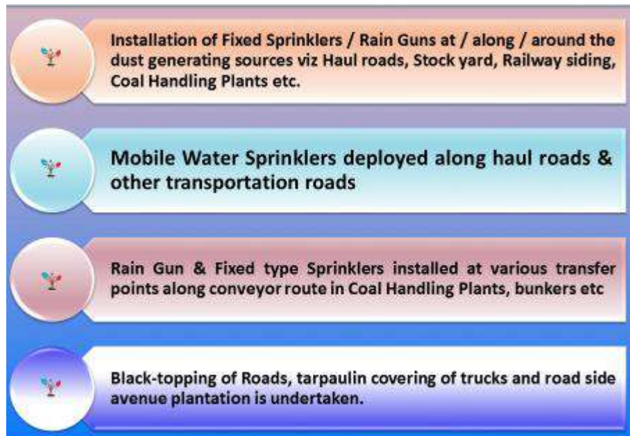
(Fig.47- Air Pollution Control Measures)
