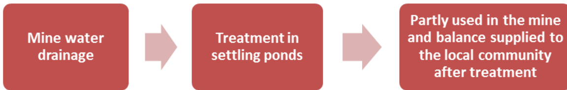
Fig. 54 -Mine water drainage system at CIL
