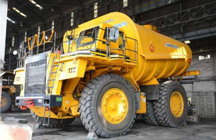
Fig.52- NCL has commissioned a mobile water sprinkler with 70,000 litres capacity in its Jayant Area to suppress dust effectively. The new sprinkler can discharge 3000 litres of water up to a height of 85 metres in one minute. Assisted by hydraulic motors, the sprinkler has a higher spreading width for effective dust settling. In addition to regular features, the sprinkler also has an emergency steering and braking system, proximity warning alarm and fire-fighting unit thereby adding to the overall mine safety quotient
