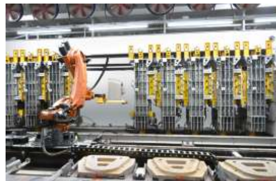
Sanitaryware Robotic Pressure Casting For producing clone type product every time
