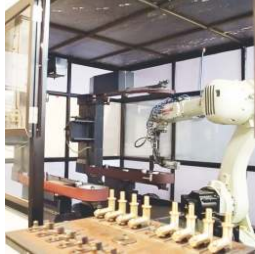
Faucet Robotic Surface Grinding Helps in uniform coat of chromium plating which leads to greater surface endurance
