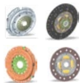
Hysteresis controlled clutch cover for AMT application in heavy commercial vehicles (430mm dia) and (362mm dia) and passenger vehicles (190mm dia)
