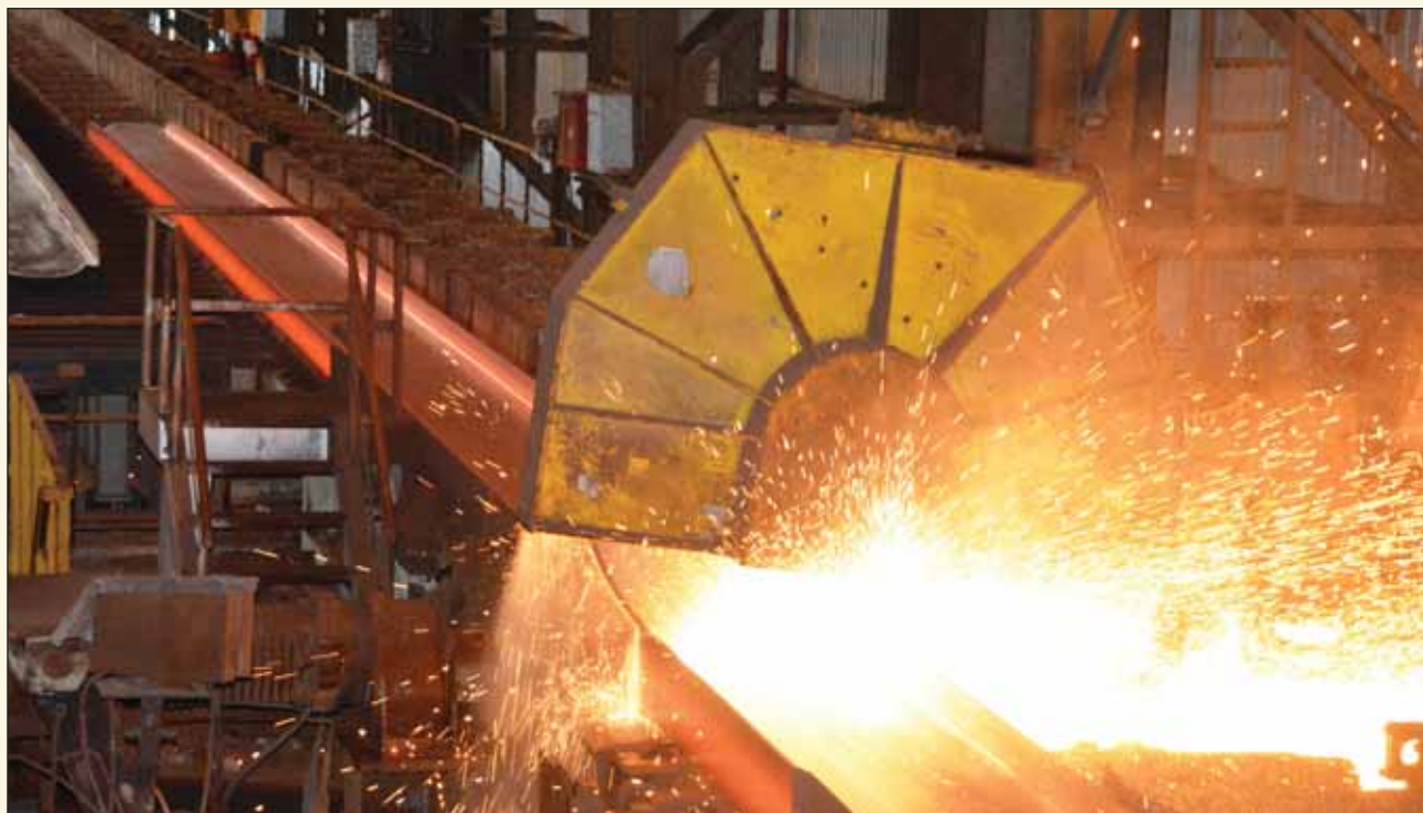
Steel Authority of India Ltd. became the first domestic steel maker to successfully roll NPB-750 (NPP-750) Narrow Parallel Flange Beams. The Beams are being rolled at new and state-of-the-art Universal Structural Mill of SAIL's IISCO Steel Plant.
