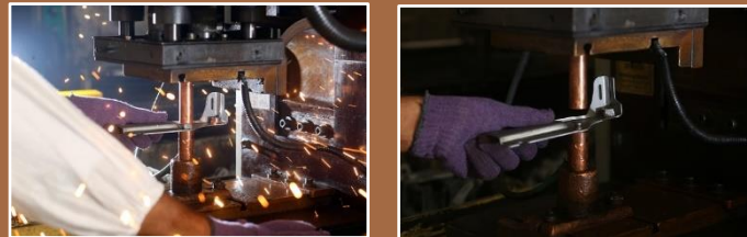
Projection Nut Welding
