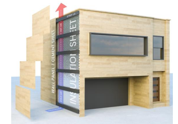
Thermal Insulation and Vent
