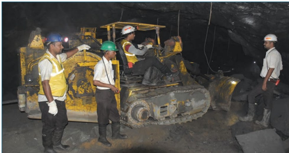
Side Dump Loader at MOIL's Mine
