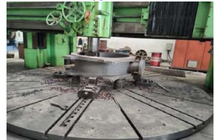
Machining of Valve outer casing.
