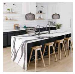
a composite material manufactured using quartz as the major raw material and has a striking resemblance in appearance to natural stone but more uniformity in colour and patterns as compared to natural stone.
