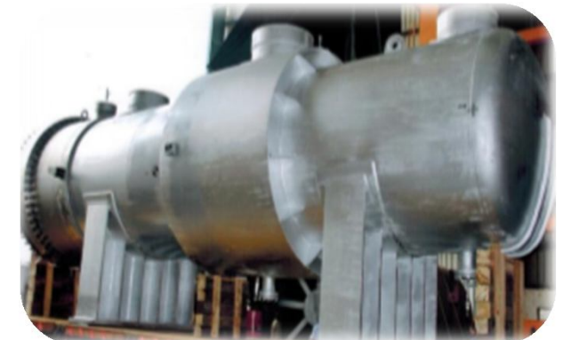
Moderator Heat Exchanger
