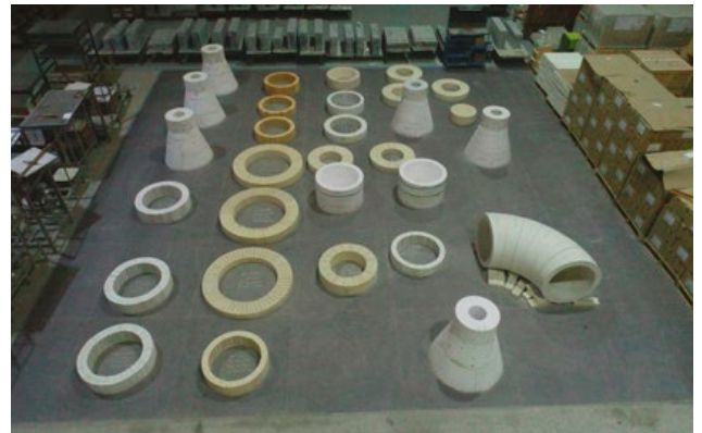
Carbon Black Reactor Refractory Lining (pre-despatch assembly) is made of high alumina refractory with low impurity. This helps customers run their reactor trouble-free to a temperature close to 2000° C.
