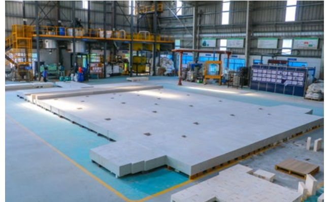
Bottom Block Refractory (pre-despatch assembly) for solar glass furnace. These blocks are precision finished with all six faces ground to tight tolerances providing a near zero gap when assembled.
