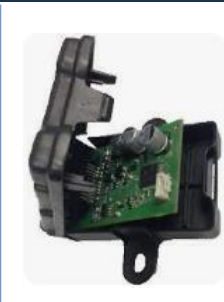
Light Control Unit
