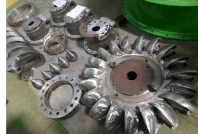
TURBINE EQUIPMENT ASSEMBLY SUNDARIJAL HYDRO PROJECT, NEPAL
