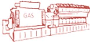
Gas - Up to 25 MVA
