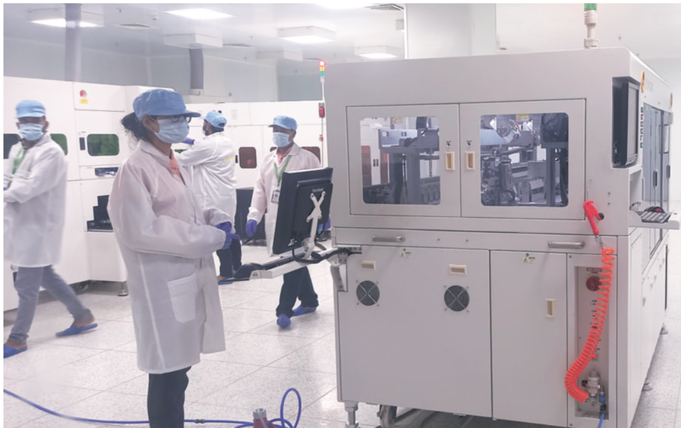
The chip assembly plant at Sahasra's factory in Bhiwadi is capable of packaging six- to 12-inch wafers
