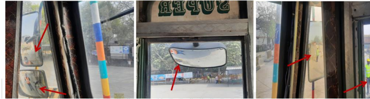
Reduce Blind Spot – After Adjusting of Mirrors
